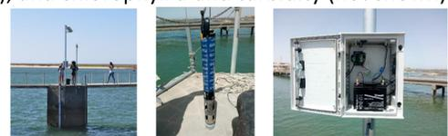
Fig. 2. RTO location, multiparametric probe with sensors and datalogger
