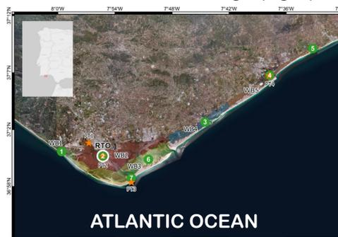
Fig. 1. Location of Ria Formosa, on south coast of Portugal, sampling stations, deployment of Pressure Transducers (PT) and real time observation station (RTO), and the limits of the water bodies (WB) identified by different colors.
