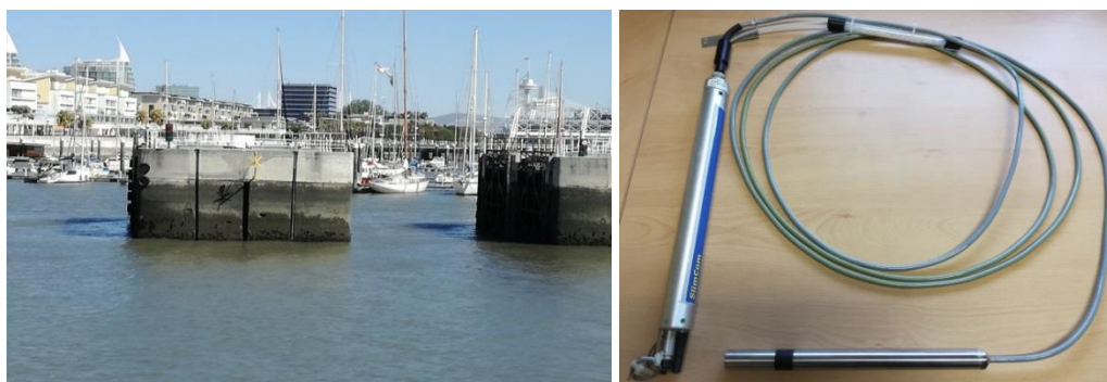
Figure 4.12 – General overview of the Parque das Nações station and SEBA MPS D3 multiparameter probe with SEBA Slimcom2 data logger
